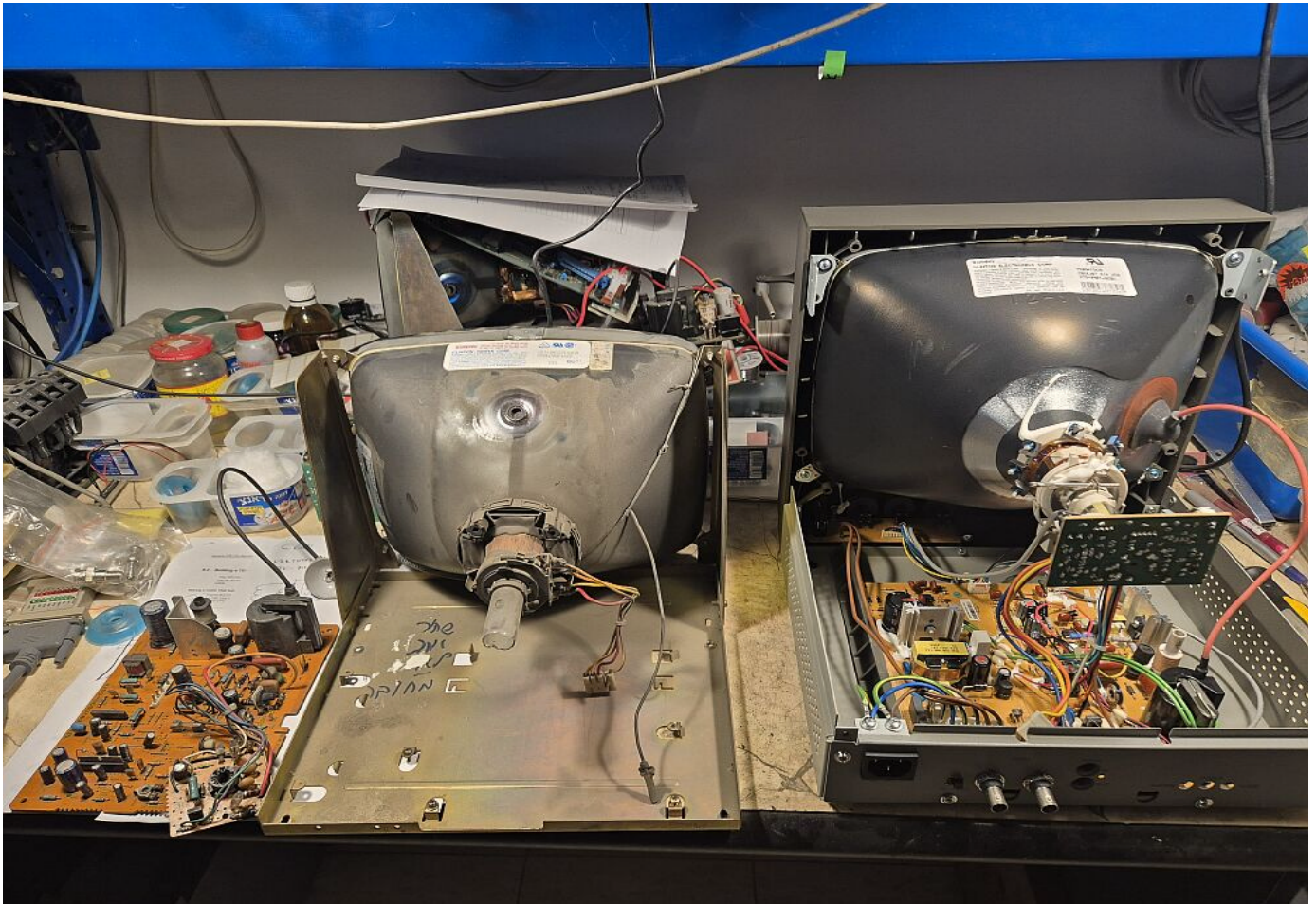
▲ A Reverse Engineered CRT Monitor while replacing its broken CRT tube.
